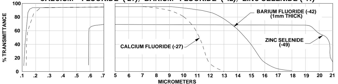
this filter does not have an anti-reflection coating and thus has transmission around 50%. Also see the -32 filter.
