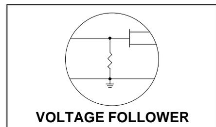
Detectors with a **voltage follower** offer a low output impedance and a high signal-to-noise ratio. The units are composed of a sensing element, an ELTEC thick-film high megohm load resistor and a field
