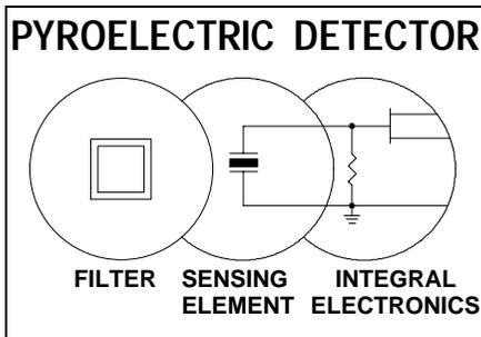
A detector consists of a **filter**, a **sensing element**, and **integral electronics**. The filter restricts incoming radiation to a wavelength band of interest, the crystal responds to the incident energy and produces a signal, and the integral electronics assist in mating the signal with other equipment. ELTEC makes available a variety of filters, crystals, and electronics so as to best meet the needs
