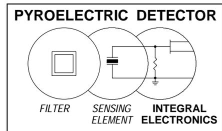
Thus to produce a more practical low-impedance voltage signal, electronics are packaged within most pyroelectric detectors. Naturally, the impedance conversion can be accomplished outside the detector, but most users choose integral electronics for reasons of convenience, reliability, shielding and cost.
