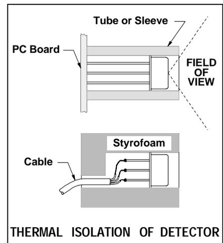
First, the instrument or device using the detector should have a completely closed housing - with plastic or laminated metal
