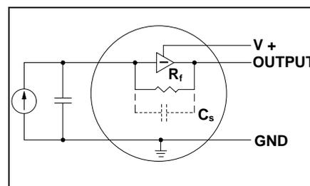
same distance but at diverse speeds. The gain is dependent on the feedback resistor,  $R_f$ . Frequency response is limited by the low pass filter ( $R_f$  and  $C_s$ ).
