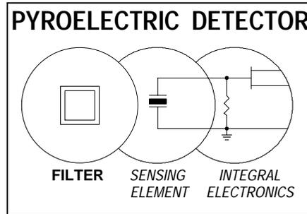
The filter protects the crystal and internal electronics from physical damage and air drafts. The filter, when properly selected, will block wavelengths of no interest and pass those desired.
