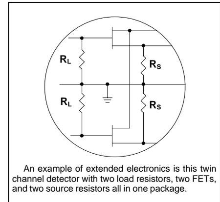
An example of extended electronics is this twin channel detector with two load resistors, two FETs, and two source resistors all in one package.
