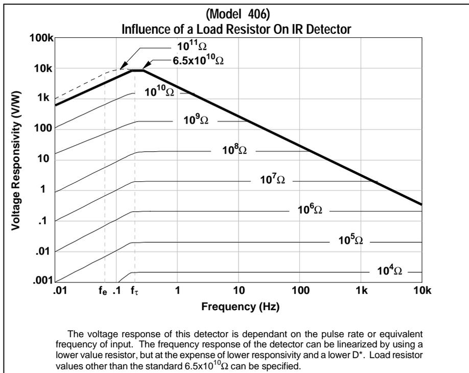
effect transistor. The thermal time constant of the crystal establishes the potential low frequency response. This thermal limit in conjunction with the effective capacitance of the sensing element (including stray) and the high megohm load resistor determine the detector's frequency response. As the sample curve shows, responsivity decreases as load resistors are chosen to extend flat response.
