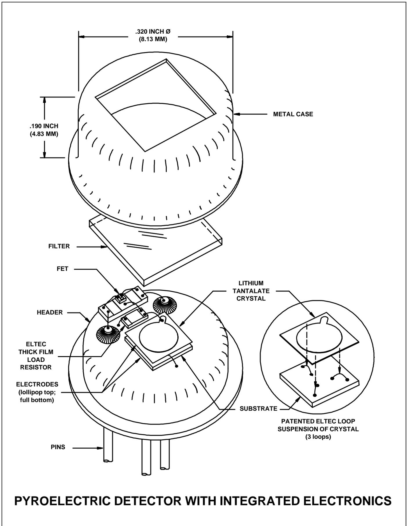
Figure 3. Single-element lithium tantalate detector with detail of crystal suspension.
