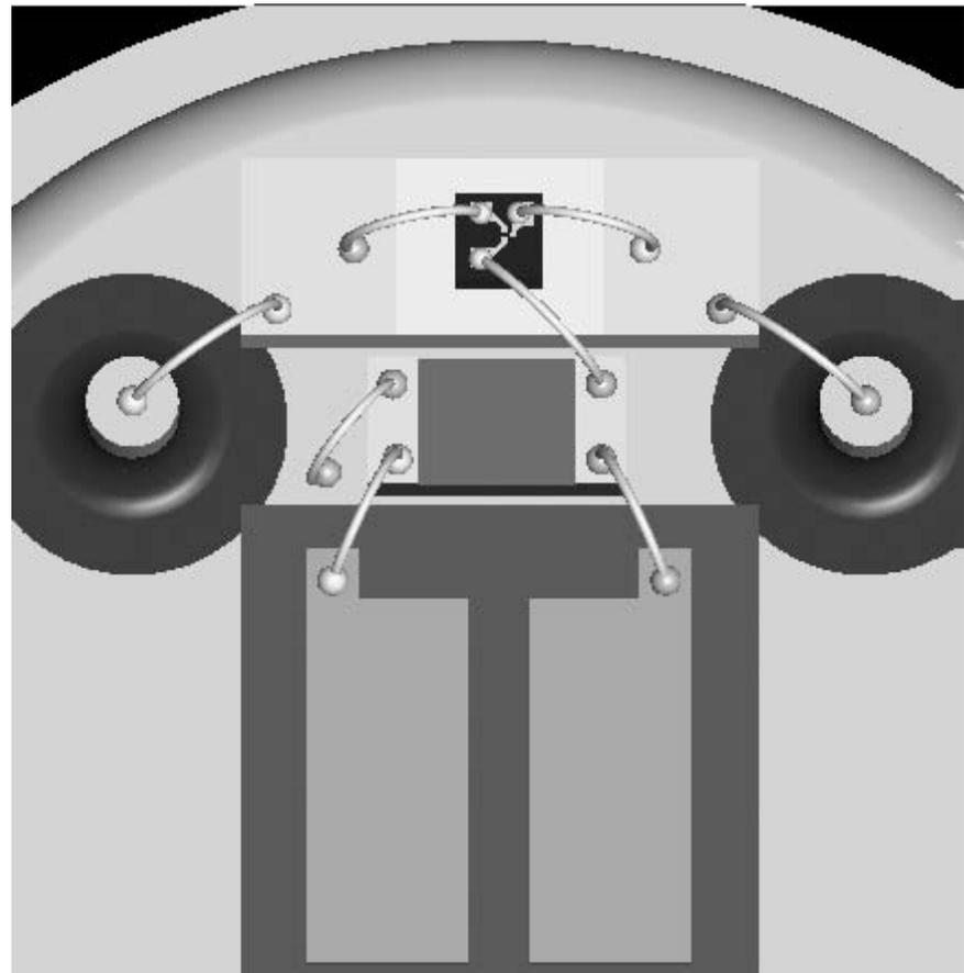
Figure 10. Header of dual element, series opposed lithium tantalate detector with load resistor and FET. Bottom electrode unconnected (floating). Wire from resistor to header makes case ground. Graphic enhanced to make 0.025mm (1 mil) gold wire visible.
