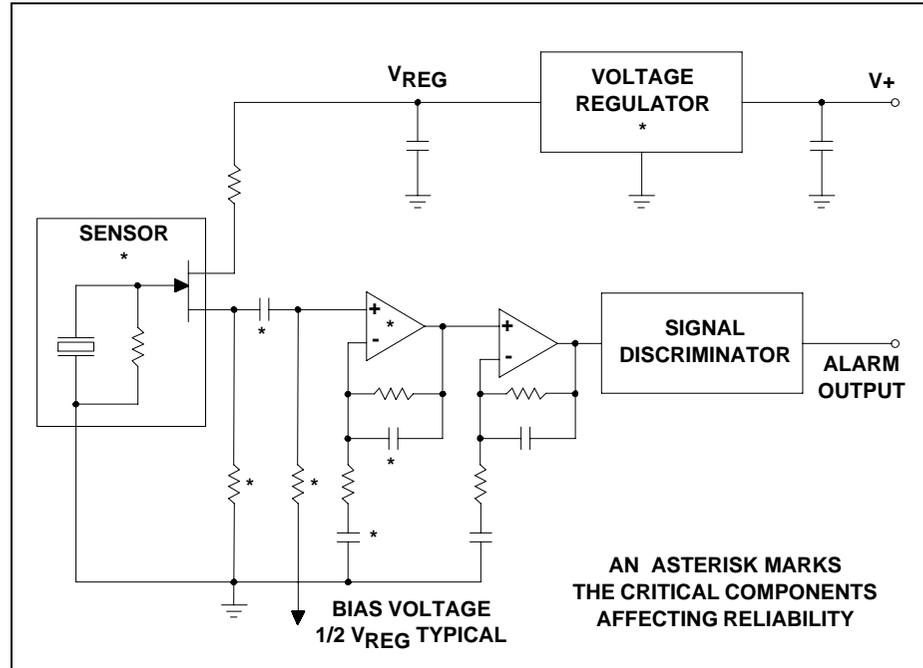
Figure 5. Typical intruder alarm circuit.
