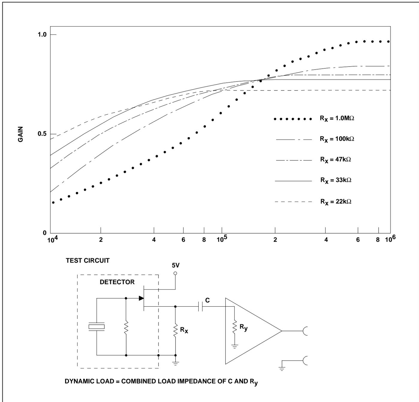
Figure 4. Impedance converter FET gain versus load (or "source") resistor and dynamic load.
