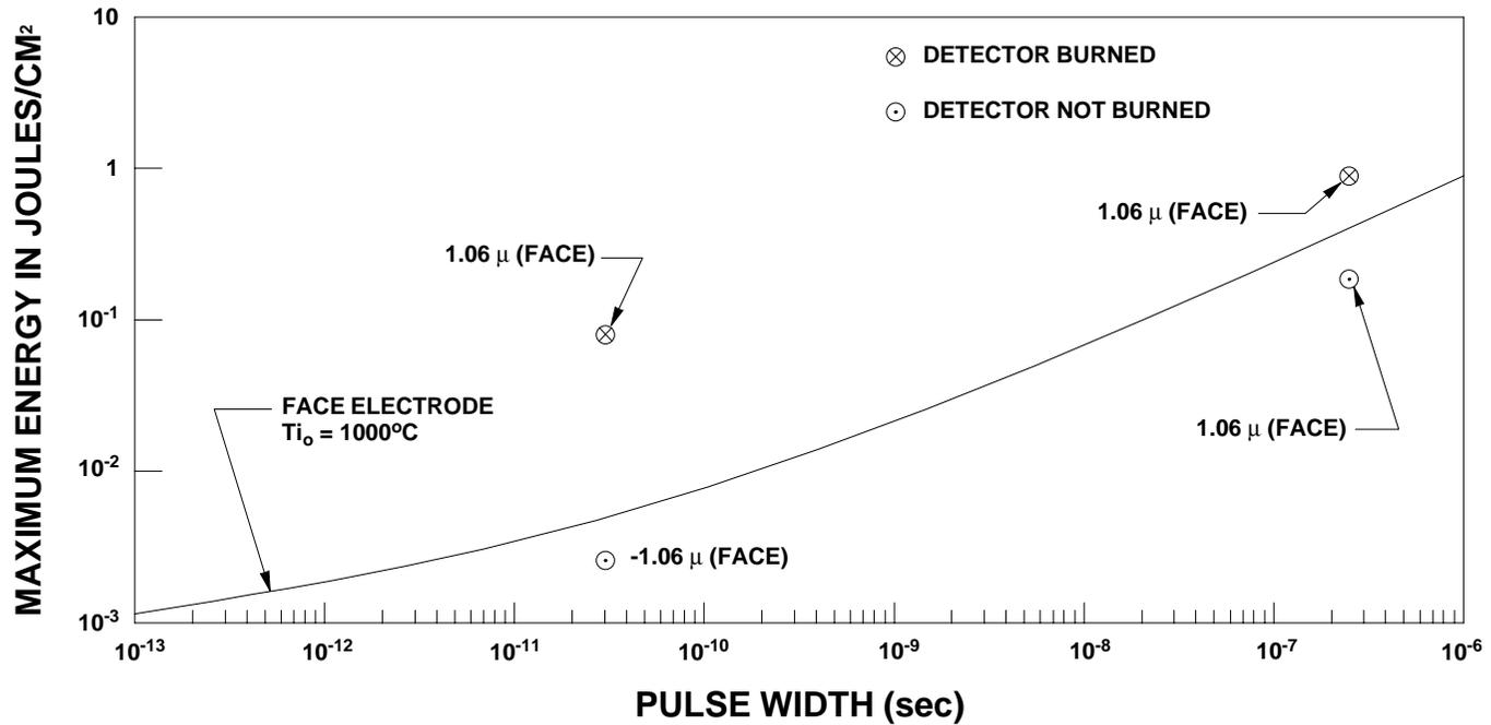
Survivability of face electrode pyroelectric detectors to high speed laser pulses. Detectors can tolerate greater energy from longer pulses because energy has time to dissipate through the sensing crystal rather than simply bringing electrode material (very thin) to damage level. Data is from pages 37 - 38 of "Advances in Pyroelectric Detectors", doctoral dissertation by Carlos Roudy for Stanford University, 1972. See also ELTECdata # 109, page 2.
